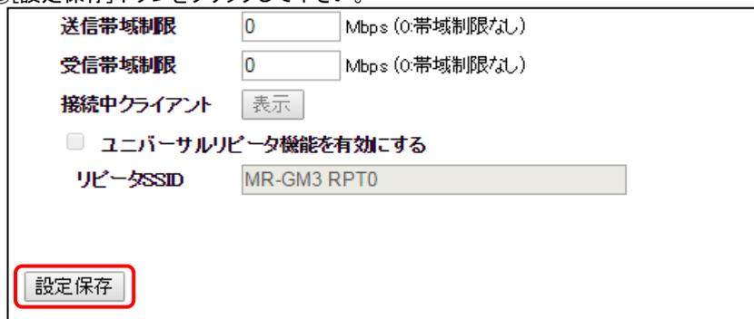
This is the 'Advanced Settings' page for wireless LAN. It contains several fields: '送信帯域制限' (Transmit bandwidth limit) set to '0' Mbps, '受信帯域制限' (Receive bandwidth limit) set to '0' Mbps, and a '接続中クライアント' (Connected clients) section with a '表示' (Show) button. There is an unchecked checkbox 'ユニバーサルリピータ機能を有効にする' (Enable universal repeater function) and a 'リピータSSID' (Repeater SSID) field set to 'MR-GM3 RPT0'. At the bottom left, the '設定保存' (Save settings) button is highlighted with a red box.
