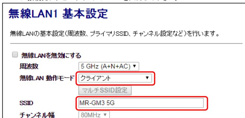
This is a zoomed-in view of the '無線LAN1 基本設定' page. The '無線LANを無効にする' checkbox is still unchecked. The '周波数' field is set to '5 GHz (A+N+AC)'. The '無線LAN 動作モード' dropdown menu is set to 'クライアント' (Client), which is highlighted with a red box. Below it is a 'マルチSSID設定' button. The 'SSID' text input field contains 'MR-GM3 5G' and is also highlighted with a red box. The 'チャンネル幅' (Channel width) field is set to '80MHz'.
