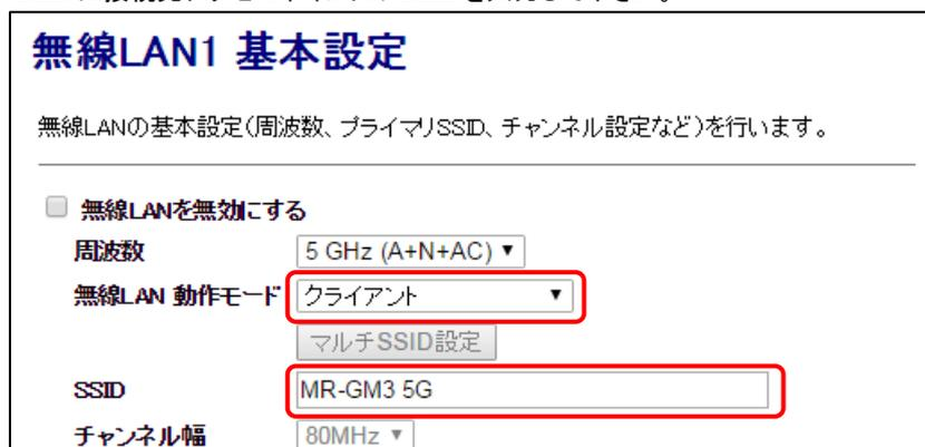
This is a close-up of the '無線LAN1 基本設定' page. The '無線LANを無効にする' checkbox is unchecked. The '周波数' dropdown is set to '5 GHz (A+N+AC)'. The '無線LAN 動作モード' dropdown is set to 'クライアント' (Client), which is highlighted with a red box. Below it is a 'マルチSSID設定' button. The 'SSID' text input field contains 'MR-GM3 5G' and is also highlighted with a red box. The 'チャンネル幅' (Channel Width) dropdown is set to '80MHz'.
